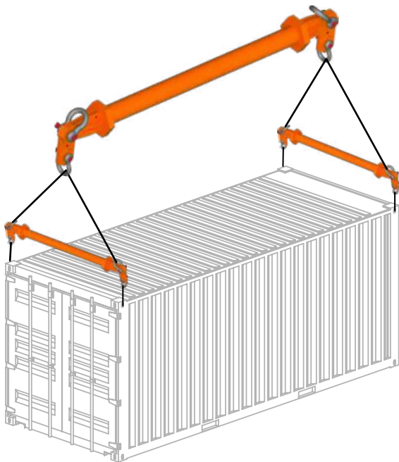
Lifting with vertical twistlocks.
