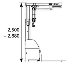
Height lifting column in mm, ready for use
