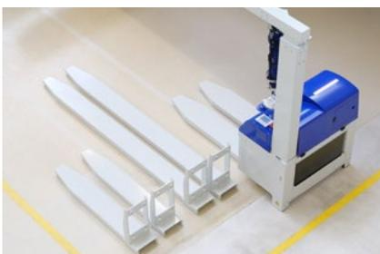
Compatible with any forklift vehicle thanks to different fork shoe variants.
