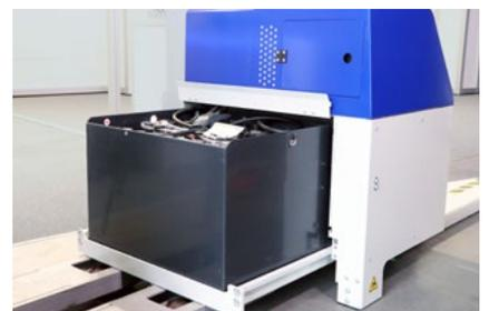
The battery can be charged in the device and also changed in approx. 10 – 15 minutes for multi-shift operation.
