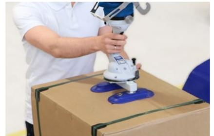
The tube lifter is started at the push of a button. It can be combined with various quick-change grippers.
