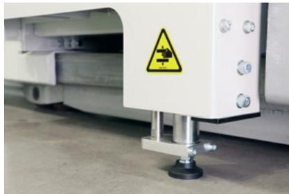
The support feet extend automatically after the jib is unlocked, minimizing cycle times.
