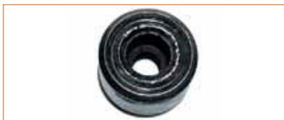
interior ring damaged for 100%
