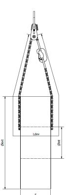
Check that the sling is correctly buckled without twisting. Check that the safety latch is closed and that the hook mouth is pointing inward. Check the space between the spool and the floor and the correct passage of the strap and fasteners to avoid jamming the parts. All accessories must be perfectly mobile in all directions without encountering any obstacle to movement.
