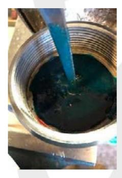
NB: At the outset the mixture has a thick, liquid consistency. It then becomes thinner until a certain point at which the hardening process begins. The Wirelock must be poured before the mixture reaches its thinnest state.
