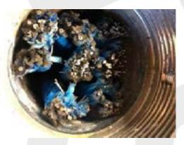
Fasten the rope so that it is vertical, while a piece (approx. 25 x d) of the rope is hanging vertically. Pack the base of socket with e.g. putty to prevent any Wirelock escaping during the sealing process.
