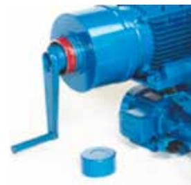
MANUAL EMERGENCY CRANK (ON ELECTRIC MOTOR)
